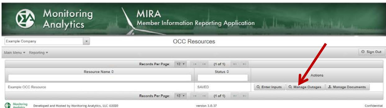
On the Manage Outages screen, select the plant or unit that will be out, the start and end date of the outage, and the Operating Percent for the outage period.
