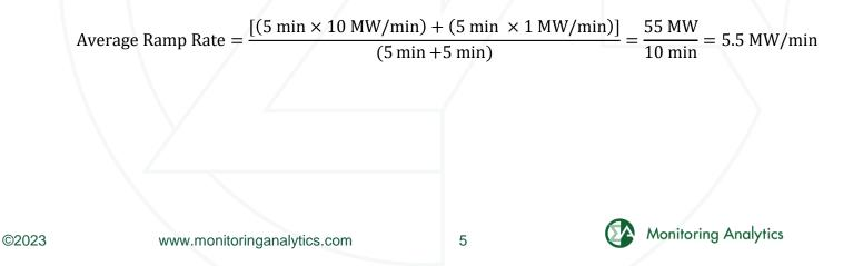
The 5.5 MW/min ramp rate is used in the synchronized reserve (SR) MW capability calculation. This unit SR MW will be limited by 5.5 MW/min times 10 minutes, or 55 MW. The unit can provide 100 MW of SR reserves when operating between 300 MW and 400 MW. Beyond 400 MW, the unit's SR capability is reduced because the ramp rate goes down to 1 MW/minute after 500 MW.
