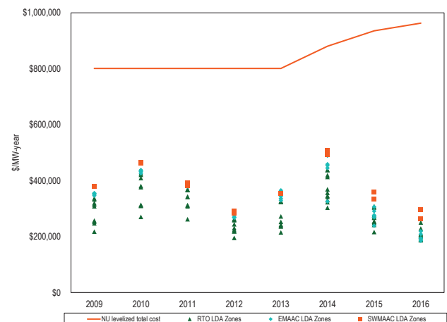
Figure 7-9 New entrant NU net revenue and 20-year levelized total cost by LDA (Dollars per installed MW-year): 2009 through 2016
