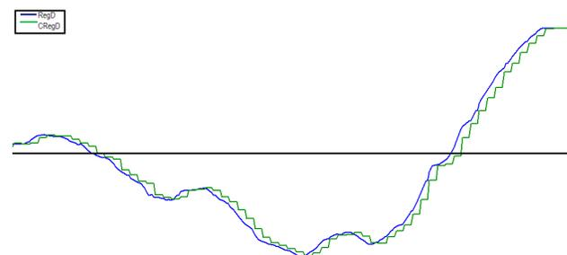
Regulation signals are designed for the purpose of moderating ACE, accounting for the characteristics of the expected response from the resources following the signal. The RegD signal is designed to contribute to the moderation of ACE given the attributes of fast regulation resources. The RegA signal is designed to contribute to
