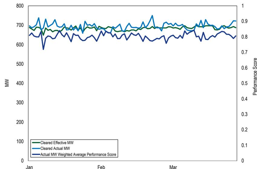
In Figure 10-3 and Figure 10-4, actual MW are unadjusted for either performance score or benefit factor and effective MW are adjusted for the historic 100-hour moving average performance score and the resource-specific benefit factor.
