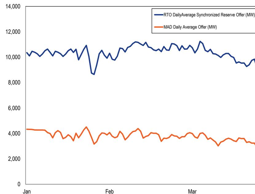
Synchronized reserve is offered by steam, CT, CC, hydroelectric and DR resources. Figure 10-14 shows average offer MW volume by market and unit type for the MAD subzone and Figure 10-15 shows average offer MW volume by market and unit type for the RTO Zone.
