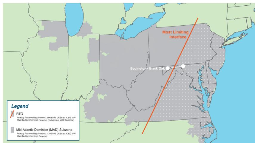
Of the 2,063 MW RTO primary reserve requirement, PJM requires that at least 1,375 MW be synchronized to the grid. The synchronized reserve requirement is 100 percent of the largest contingency. Of the 1,375 MW of synchronized reserve requirement for the RTO, 1,300 MW must be deliverable to the Mid-Atlantic Dominion Subzone.
