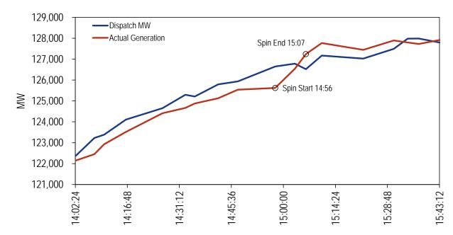
Figure 1 October 1, 2019 RT SCED Dispatch MW and Actual Generation during low ACE event.
