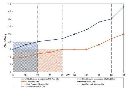
In case of dual fuel units, if the price-based offer uses a cheaper fuel and the cost-based offer uses a more expensive fuel, the price-based offer will appear to be lower cost even when it includes a markup. Figure 3-60 shows an example of offers by a dual fuel unit, where the active cost-based offer uses a more expensive fuel and the price-based offer uses a cheaper fuel and includes a markup.
