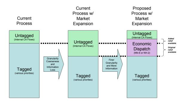
**Market Flows** are defined as the flows generated from an operational entity's dispatch, and is equal to the sum of firm and non-firm flows. The firm components consist of the flows created both through serving Network Native Load (NNL) and by those schedules flowing on Firm transmission reservations (7-F). For the purposes of this proposal, both firm transmission and NNL schedules will be referred to as the **NNL** component of Market Flows, and are considered firm.
