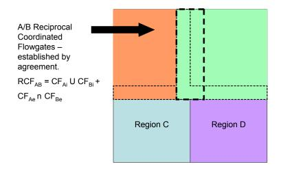
If C wished to enter into a reciprocal coordination agreement with A, C would have to first establish their own set of Coordinated Flowgates. Following this, they would identify the set of Reciprocal Coordinated Flowgates, then agree to coordinate operations based on the flowgates contained in that that set
