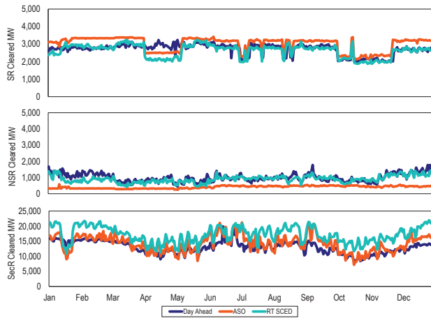
Figure 10-3 MW cleared by the day-ahead engine, the ASO, and RT SCED: 2024
