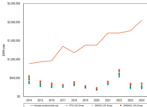
Figure 7-8 New entrant nuclear plant net revenue and 20-year levelized total cost by LDA (Dollars per installed MW-year): 2014 through 2024
