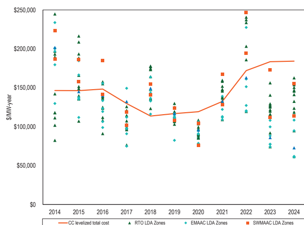
Figure 7-6 New entrant CC net revenue and 20-year levelized total cost by LDA (Dollars per installed MW-year): 2014 through 2024
