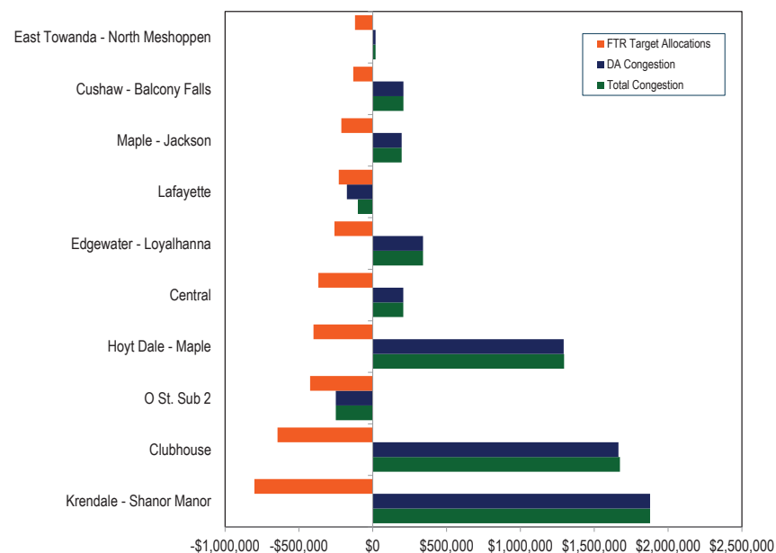
Figure 13-18 Top ten constraint sources of negative FTR target allocations: June 2022 through May 2023
