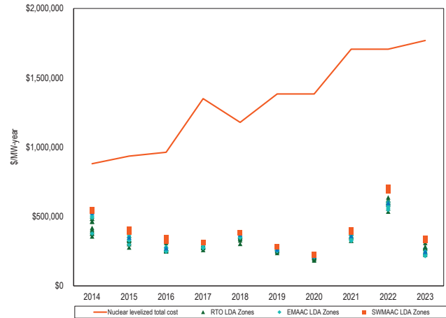
Figure 12 New entrant nuclear plant net revenue and 20-year levelized total cost by LDA (Dollars per installed MW-year): 2014 through 2023
