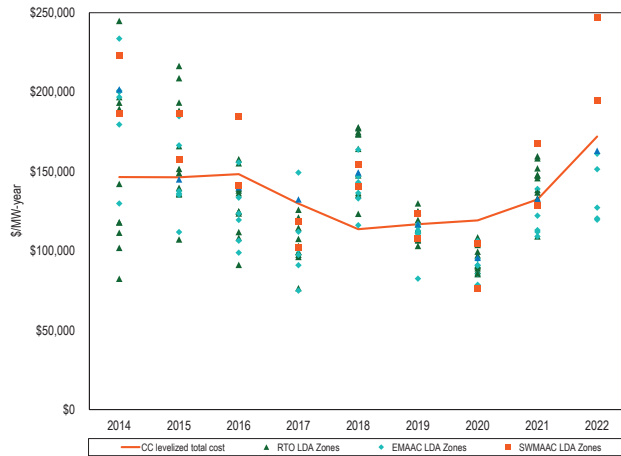
Figure 10 New entrant CC net revenue and 20-year levelized total cost by LDA (Dollars per installed MW-year): 2014 through 2022
