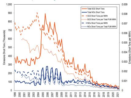
Figure 8-12 SO<sub>2</sub> and NO<sub>x</sub> emissions by quarter (thousands of short tons), by PJM units: January 1999 through June  $2021^{233}$
