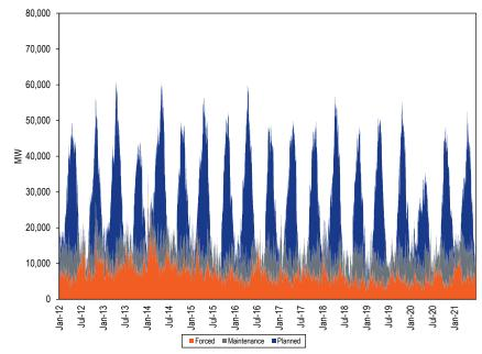
In 2020, planned, maintenance and forced outages were lower than in 2019 (Figure 5-11). The MWh of planned outages were 26 percent lower than in 2019. The MWh of maintenance outages were 7 percent lower than in 2019. The MWh of forced outages were 20 percent lower than in 2019. In 2021, planned outages were 15 percent lower, maintenance outages were 9 percent
