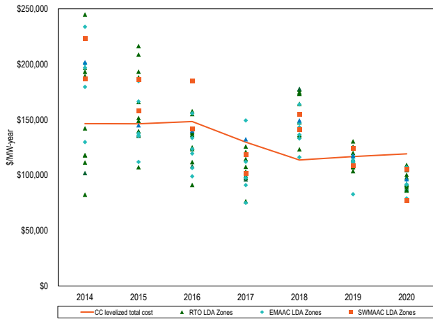
Figure 12 New entrant CC net revenue and 20-year levelized total cost by LDA (Dollars per installed MW-year): 2014 through 2020
