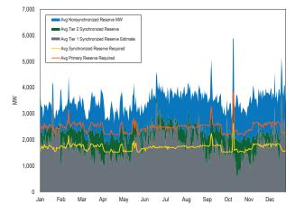
Figure 10-2 shows that within the MAD Subzone, Tier 1, Tier 2 from MAD, and Tier 2 from the RTO are all essential to satisfying the synchronized reserve requirement. Figure 10-3 shows that tier 1 synchronized reserve remains the major contributor to satisfying the synchronized reserve requirement in the RTO Zone.
