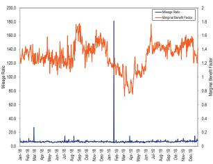
The increase in the average mileage ratio caused by the signal design changes introduced on January 9, 2017, caused a large increase in payments to RegD resources on a performance adjusted MW basis.
