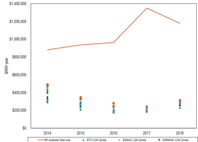
Figure 15 New entrant NP net revenue and 20-year leveled total cost by LDA (Dollars per installed MW-year): 2014 through 2018
