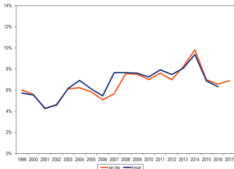
Figure 5-11 Trends in the PJM equivalent demand forced outage rate (EFORd): January 1 through September 30, 1999 through 2017
