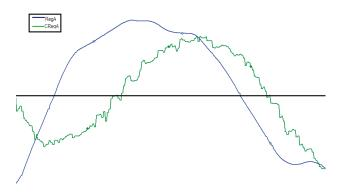
Figure E-6 PJM RegD signal and CRegD current regulation signal. Example of typical 10-minute time period
