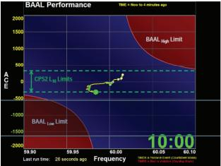
PJM counts the total number of minutes that ACE complies with the BAAL limits (high and low) and divides it by the total number of minutes for a month, with a passing level for this goal being set at 99.0 percent for each month. BAAL high and low limits are defined dynamically.<sup>9</sup>
