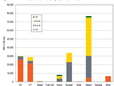
Figure 12-2 PJM capacity (MW) by age (years): At September 30, 2015
