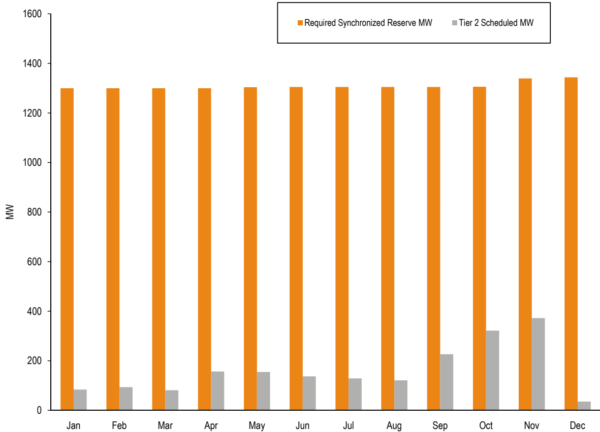
Figure 10 RFC Synchronized Reserve Zone monthly average synchronized reserve required vs. Tier 2 scheduled MW: Calendar year 2008
