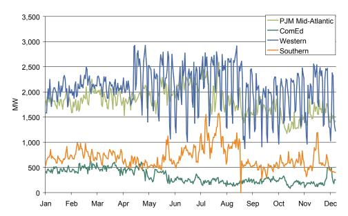
Synchronized reserve is offered by steam, CT, hydroelectric and DSR resources. Figure 6-9 shows average eligible MW volume by ancillary service area and unit type.
