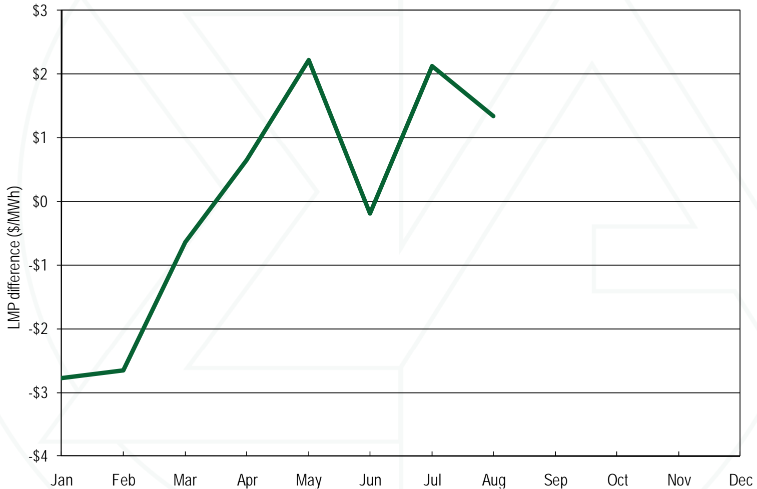
Figure 2-23 Monthly simple average of real-time minus day-ahead LMP: January through August 2010 (See 2009 SOM, Figure 2-21)
