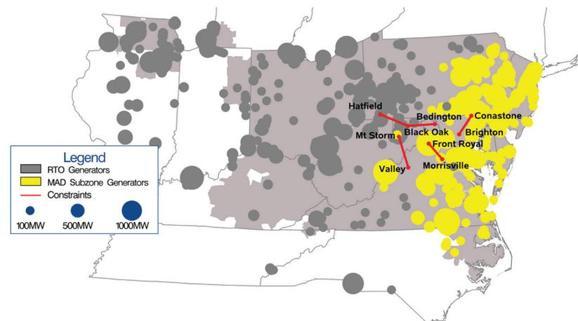
The most limiting transmission constraint for power flow from the RTO Zone into the MAD Subzone since August, 2017, has been the AP South Interface, which includes Brighton-Conastone, Belmont-Stonewall, Bedington-Black Oak, Cloverdale-Lexington, and Mt. Storm-Valley constraints.
