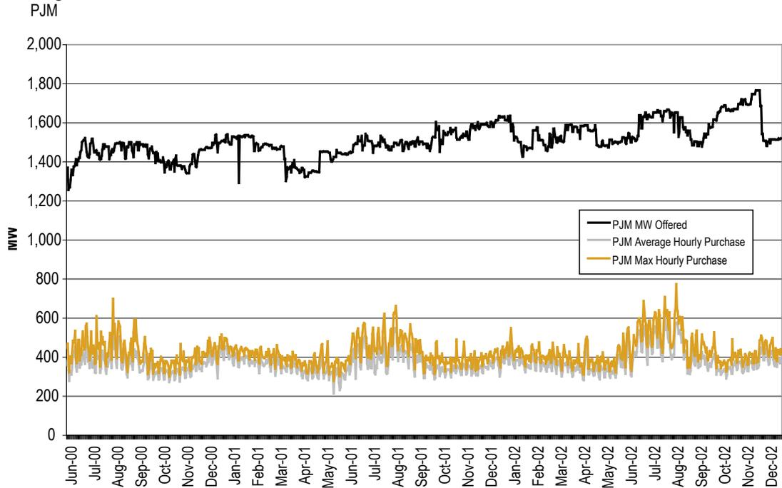
Figure 5-1b Regulation MW Offered Versus MW Purchased
